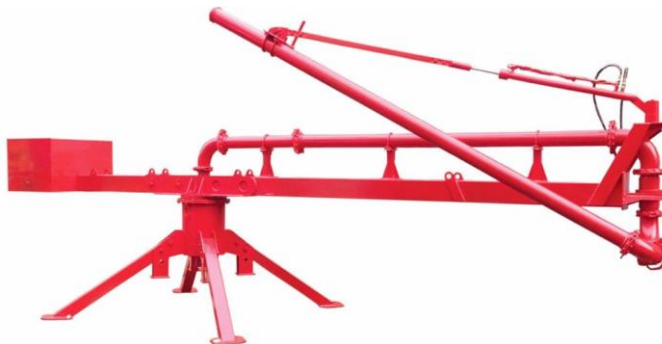
Gambar 18. Distributor/spreader dan boom
